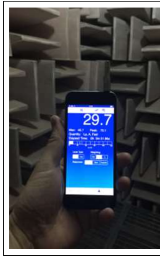
Fig. 3 Measurement in the anechoic chamber
