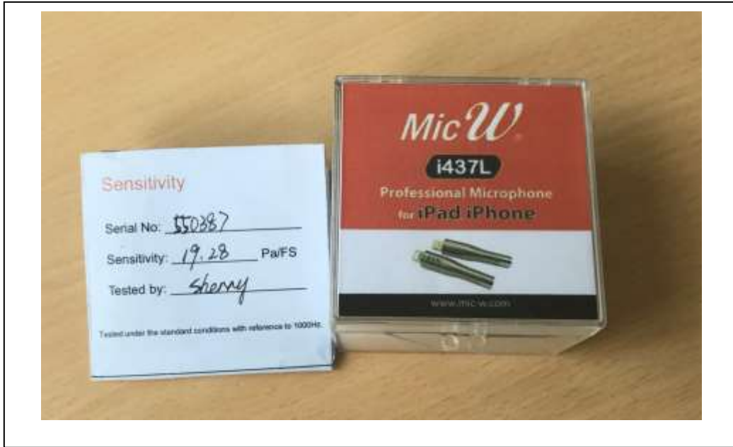
Fig 8. The calibration data supplied with each i437L with Serial Number. The sensitivity is given in Pa/FS.
