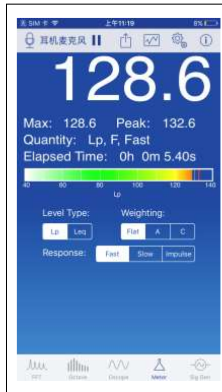
Fig. 4 Measurement setup for Maximum SPL testing. The sine signal starts the distortion when the SPL reaches 129 dB.
